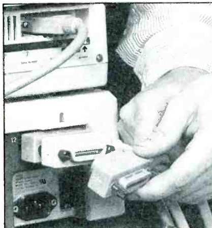
There is only one type of GPIB connector used. Most have a male and a female connector on each cable end, allowing the connectors to be stacked on top of each other.
